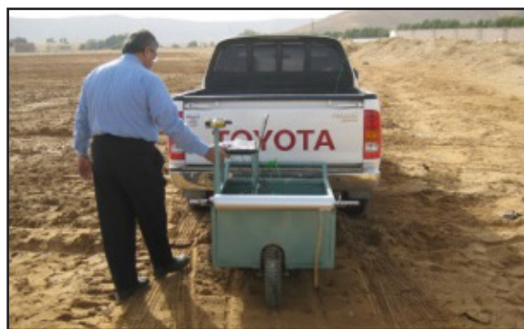
Fig. (2): A vehicle pulls the fabricated Mole carriage over the field.
